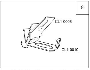
Assemble Clip CL1-008 with CL1-0010 as indicated in the above diagram. Insert tab of CL1-0008 through slot in CL1-0010.
