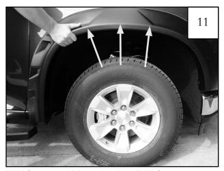
Hold flare to vehicle and re-install (3) factory screws (removed in Step 4) with a T15 bit. *Do not tighten*.
