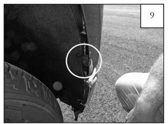
Install supplied Tab (MT1-0017) over the front location marked in Step 6. Install a clip assembly as indicated, on top of the Tab. See Step 10 for detail of clip attachment.
