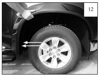
Re-install (2) factory screws (removed in Step 2) with a T15 bit. *Do not tighten*.
